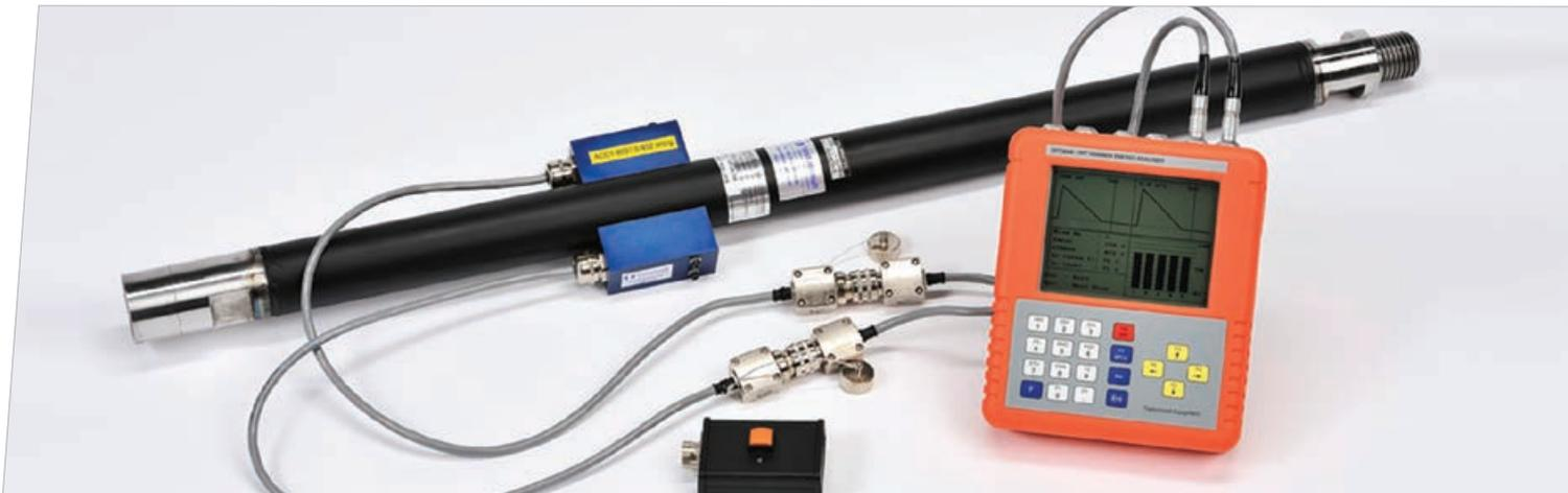
**The SPTMAN is an easy to use and portable system that is used to calculate hammer energy.**
