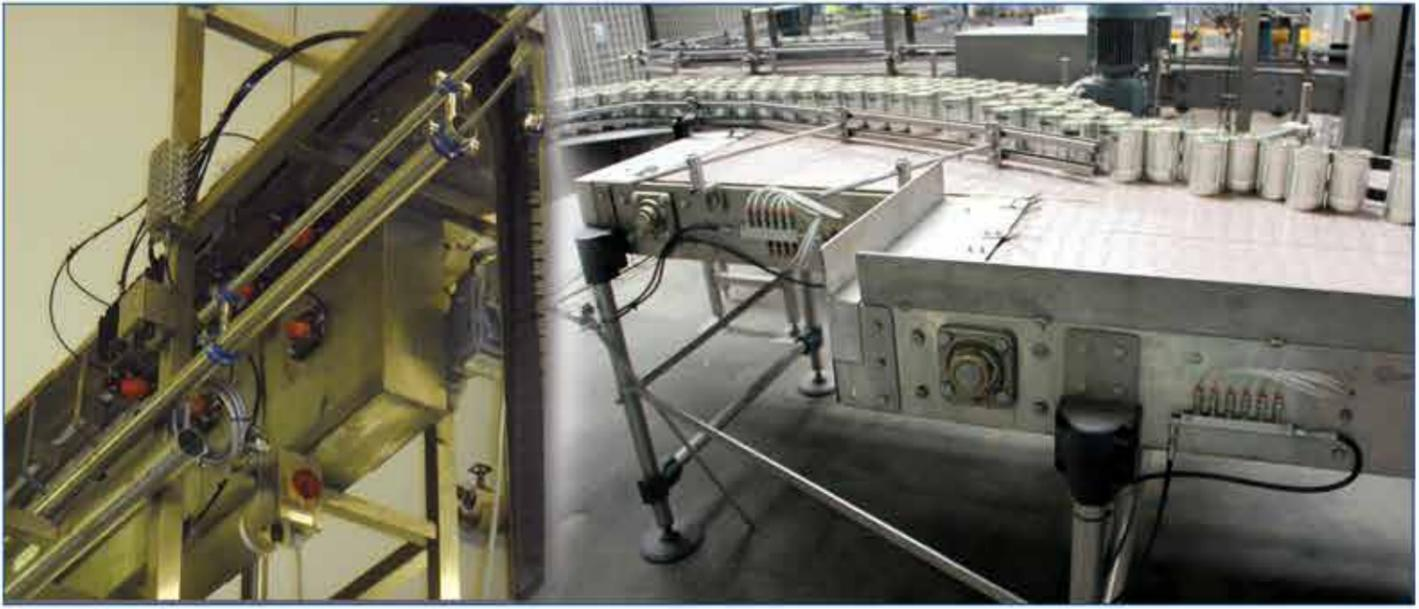
The use of lubrication systems is even more indispensable for the correct operation of machines when they operate in difficult environmental conditions, such as those in the food industry. The installation of an automatic lubrication system allows machine down times to be reduced and allows consumption of the lubricant to be controlled and the life of the bearings, chains and gears to be increased.
